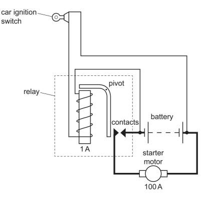
The ignition switch is in a circuit with long, thin wires. The starter motor is in a circuit with short, thick wires.
